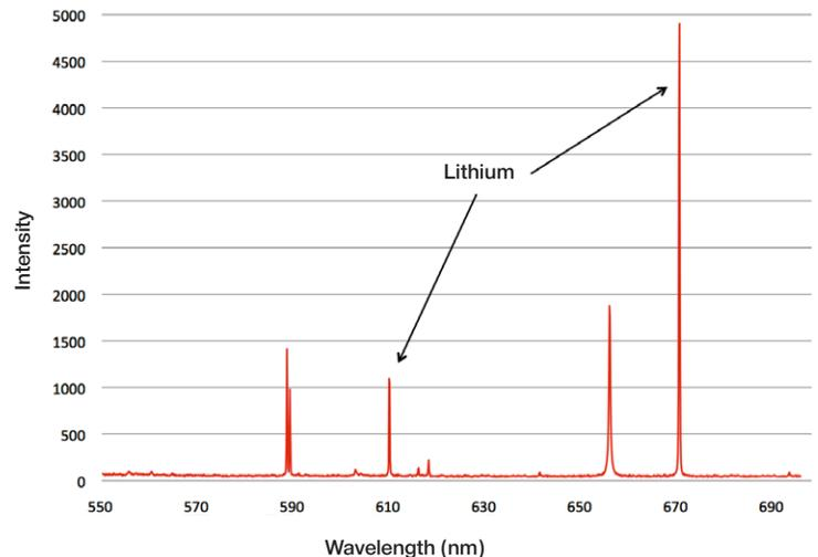
Figure 3: Spectrum from a 2 second test on a Russian manufactured aluminum alloy containing 1.86% lithium.
