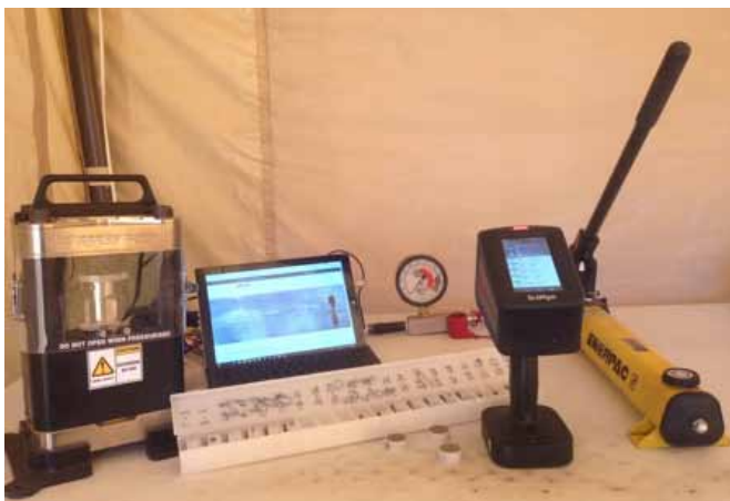
Fig. 1. Sample pelletizing using a Reflex Press and sample analyses using SciAps Z300 field-portable LIBS analyzer.
